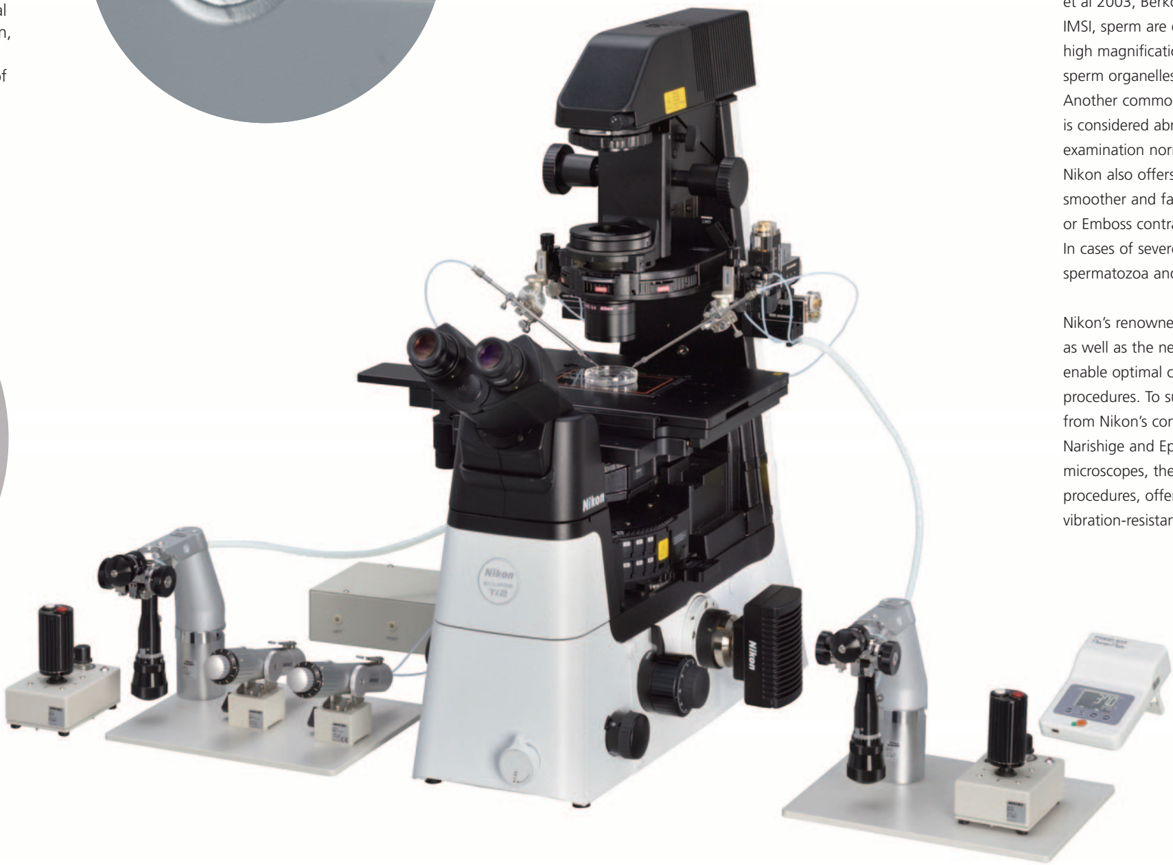
Ti2-U ICSI station with Fi3 camera
